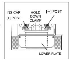
Install a new battery in the reverse order.(Always install the cable to the positive [+] post in the new battery first.)
