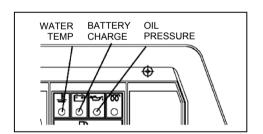
Under normal conditions, when the starter key is turned from [STOP] to [RUN], the BATTERY CHARGING and OIL PRESSURE monitor lamps will be illuminated. When the engine starts, the monitor lamps will go OFF. When a fault occurs in running, the corresponding monitor lamp will flash, and the engine will be automatically shut-off.
