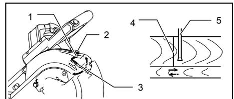
1. Screw to change the movable range of the adjusting screw
