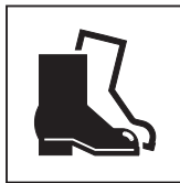
Wear Protective Footwear
