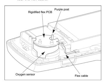
Note the placement of the PCB to ensure it is replaced correctly. Remove the two screws on the PCB.
