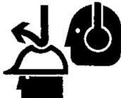
**CAUTION:** Additional Safety Protection will be required in some environments. For example, the working area may include exposure to noise level which can lead to hearing damage. The employer and user must ensure that any necessary hearing protection is provided and used by the operator and others in the work area. Some environments will require the use of head protection equipment. When required, the employer and user must ensure that head protection conforming to ANSI Z89.1 is used.
