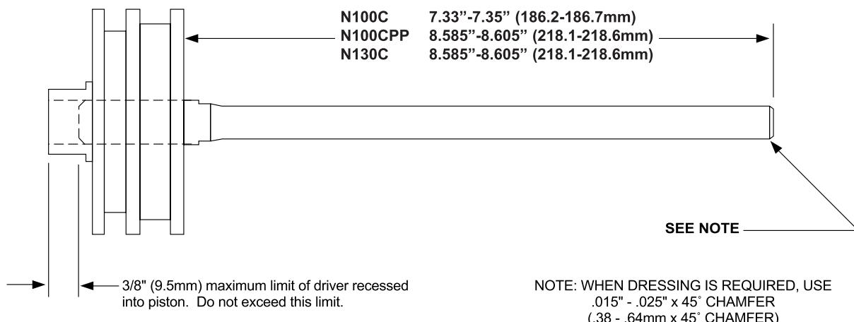
**NOTE:** Driver wear of approximately 1/8" (3mm) can be tolerated in most applications. However, in difficult driving applications, driver wear or approximately 1/16" (1.5mm) may cause a slight reduction in the apparent driving power.
