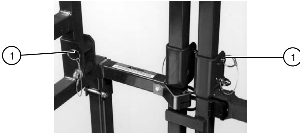
Figure 2-7. Fold-Down Guardrail System
