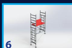
When fitting stabilisers ensure telescopic leg is adjusted to correct length. Attach top boom but leave loose enough to allow adjustment. Now attach bottom boom, again leave loose enough for adjustment. Ensure stabiliser is providing maximum footprint and firmly in contact with the ground. Once this is achieved tighten up top and bottom booms.
