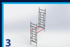
**4:** Attach 1 diagonal brace with blue trigger to the bottom rungs of each gate frame. At this point, ensure the tower is level with the use of a spirit level
